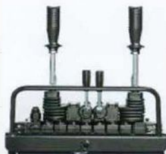
Posto guida a terra con distributore elettroidraulico. Driver's seat on the floor with electro-hydraulic distributor.
